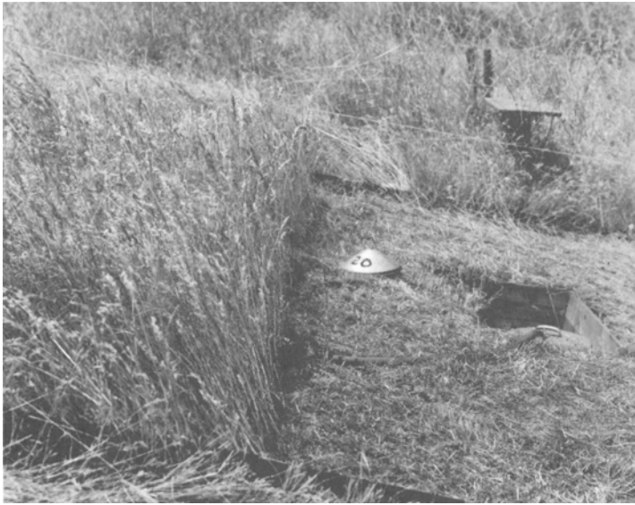
Figure 3.— Instrumentation used in the study shown by cutting away the grass at the end of a field season. A drain tube carried combined throughfall and stem-flow to the collector. A tipping bucket mechanism was used to measure rate of flow.
