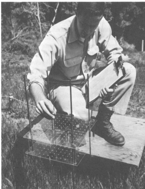
Figure 4.—A modified point-quadrat frame was used for measuring the average height of grass at the sample site and the percent of ground cover. It was also used to estimate the number of layers of vegetation available to store intercepted precipitation.
