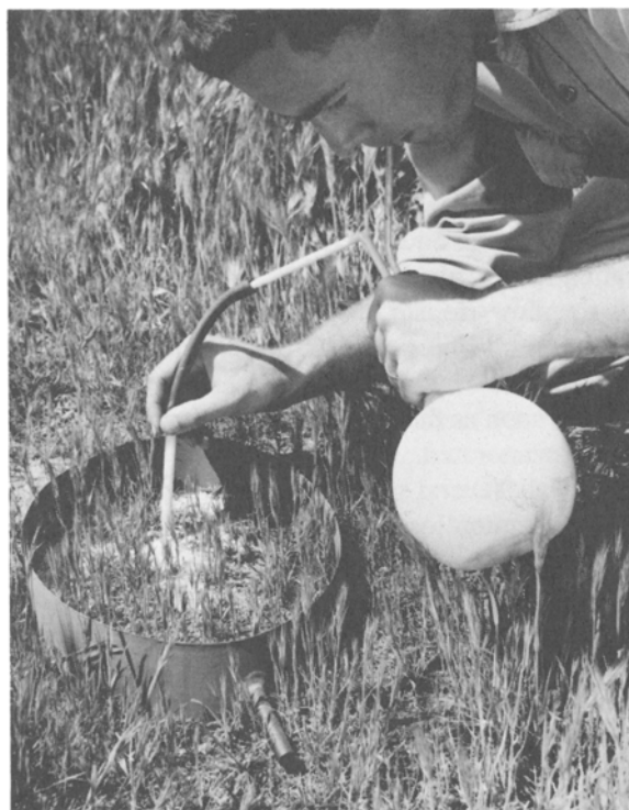
Figure 2.—Demonstration of technique used to apply neoprene sealer to soil surface inside metal collar.
