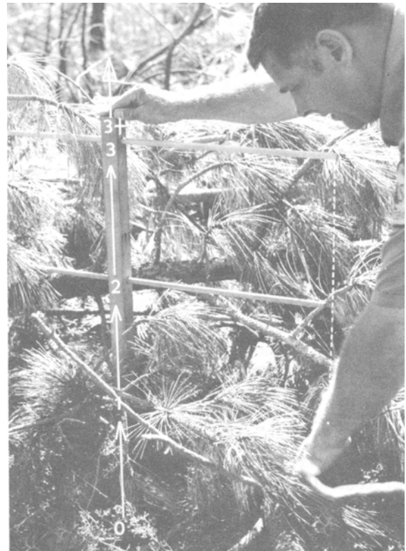
Figure 3.—A plot measuring device was used, before and after treatment, to measure fuel amount and distribution at 1-foot intervals on a vertical plane. A die was cast at each plot measuring point to determine orientation of the plane in relation to the transect line.
