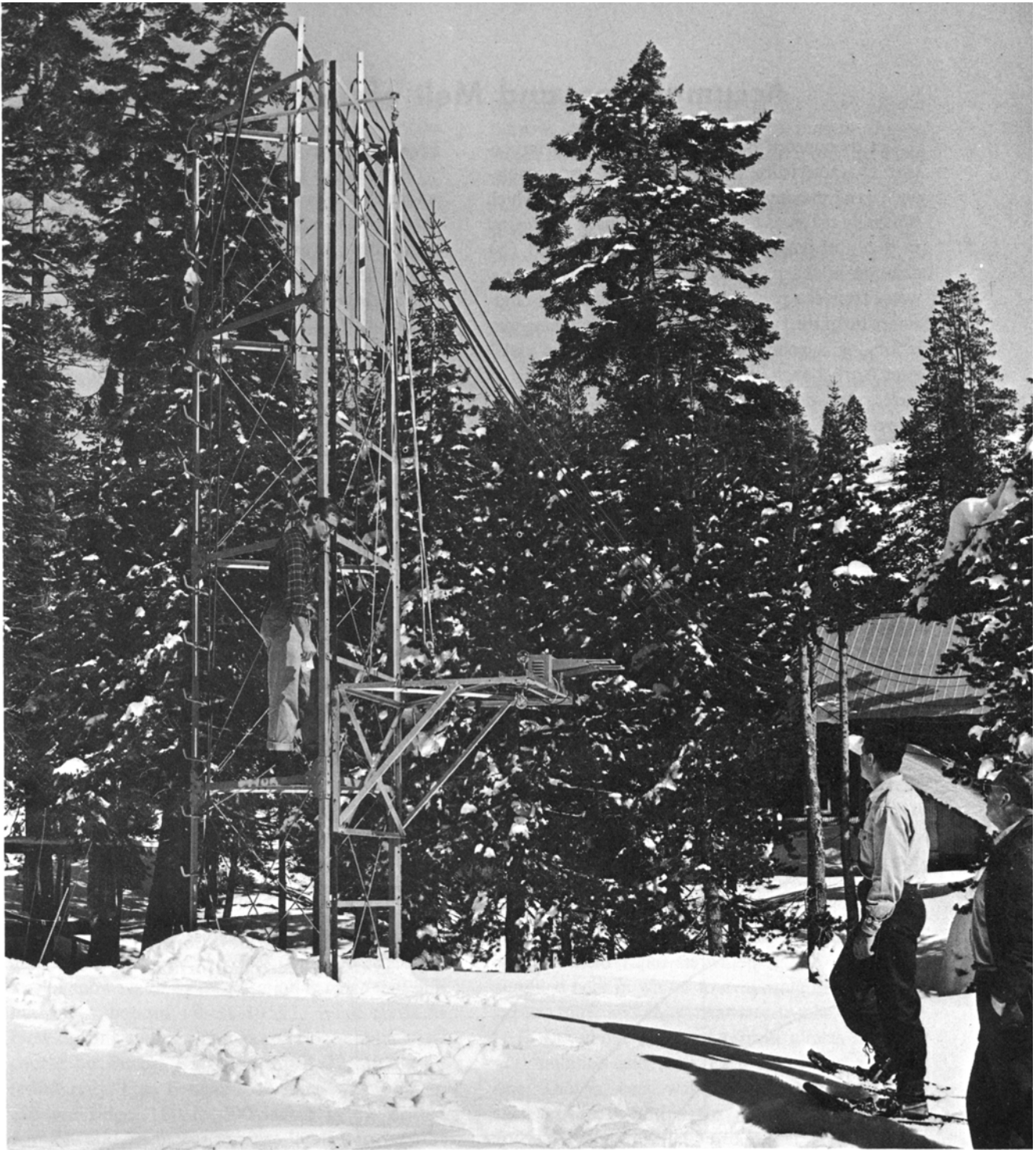
Figure 2.—Towers support meterological instruments which help evaluate moisture losses in summer and winter, snowmelt in winter, and the effects of wind, humidity, and temperature on water losses and snowmelt.
