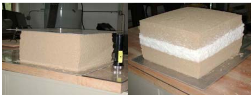
Figure 3. Pre-pressed mats with uniform wood fiber and three layer mat with chicken fiber in the core.
