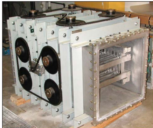
Figure 2. Microwave drying chamber showing pressing bars used for straightening curve lumbers.
