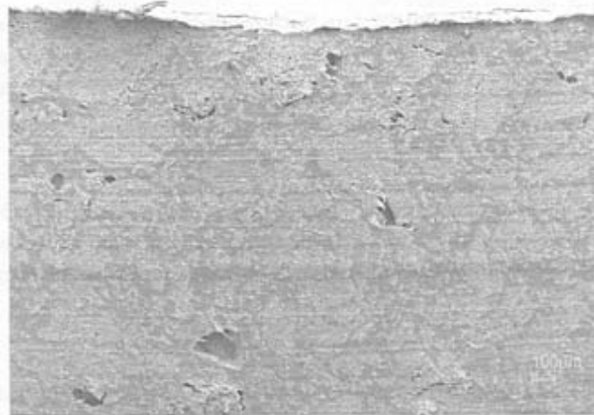
Figure 10. – SEM micrograph of a microtomed cross section of blend 3 (acetylated wood flour) without preconditioning or fungal exposure showing a few large holes (100x).
