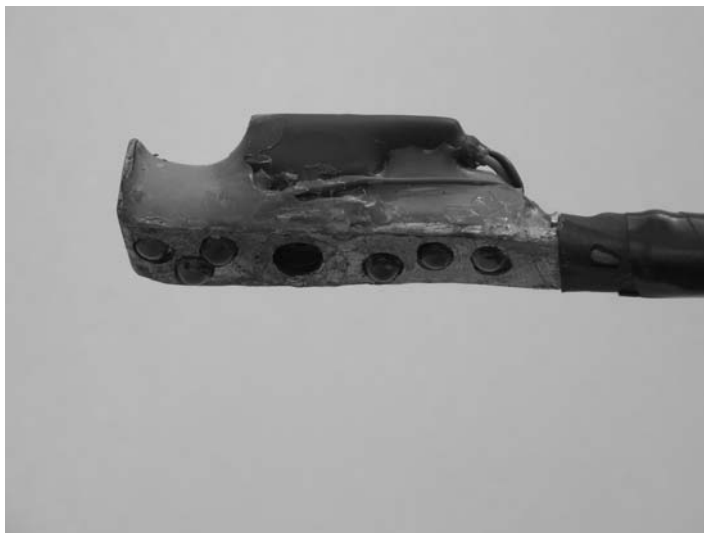
Fig. 2. Boom prepared with shelf and holes, camera and LEDs secured with hot glue.
