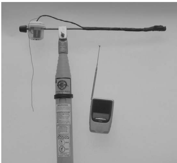
Fig. 1. Complete tree cavity viewing system, including camera boom, telescoping pole, and portable television used to examine contents of cavity nests or nest boxes.
