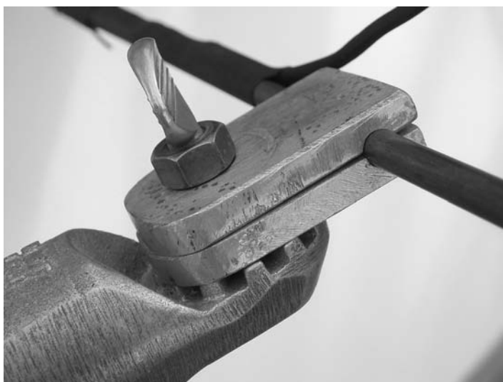
Fig. 4. Completed clamp assembly mounting the camera boom to the telescoping pole.
