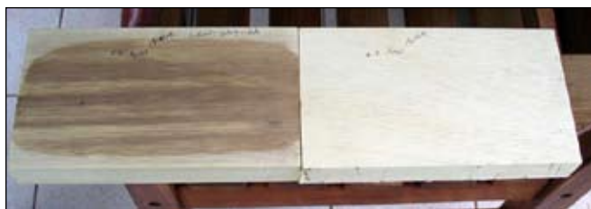
Figure 1—Ochoó boards severely affected by oxidative stain (left) and unaffected by stain (right.)
