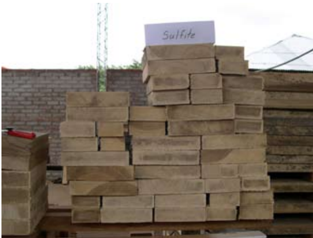
Figure 17—Cross sections of boards that were treated in sulfite solution. Note that some boards have discolored centers, others have little or no discoloration. Four of the boards are less than 50% sapwood, but their heartwood is distinguishable from discolored sapwood.
