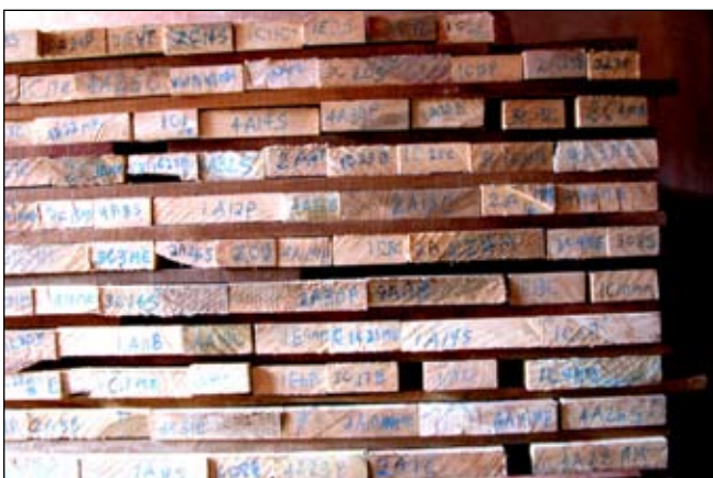
Figure 9—Sample boards in dry kiln. Tree, log, board, and treatment codes marked on ends of boards.
