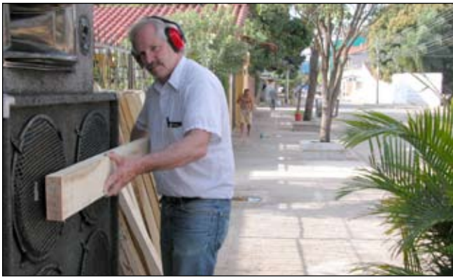
Figure 7—Board being subjected to “Reggaeton Boricua” as a vibration source.
