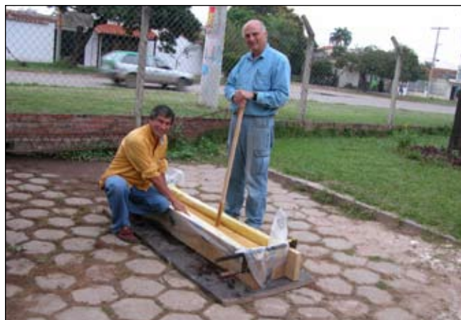
Figure 6—Board submerged in sulfite bath.
