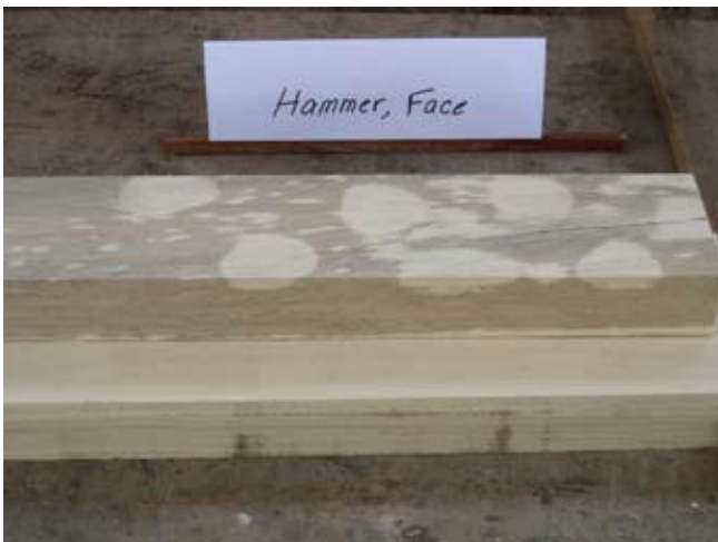
Figure 18—White marks on board surface, caused by hammer impact.
