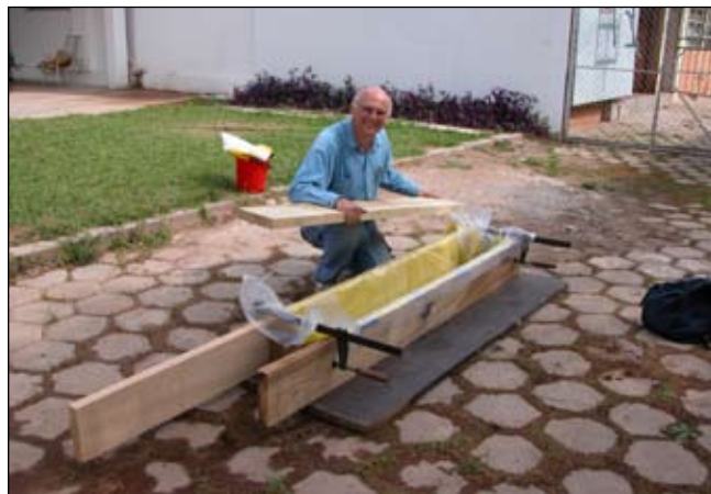
Figure 5—Basin for sulfite treatment.
