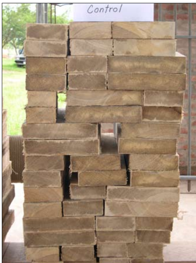
Figure 13—Cross sections of control boards, showing extensive discoloration.
