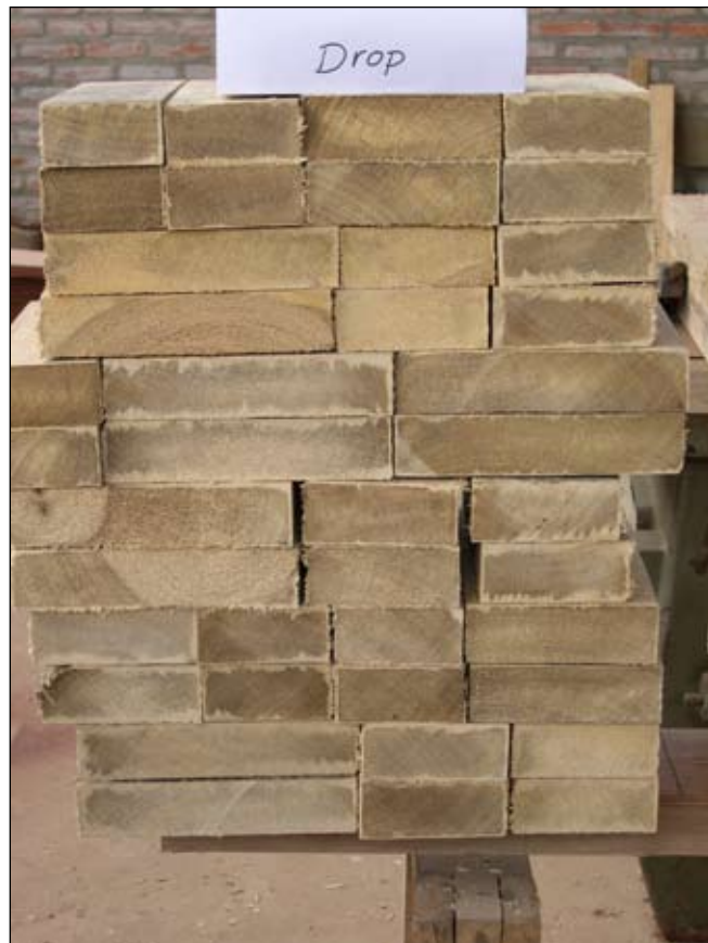
Figure 14—Cross sections of boards that were dropped on walkway to induce shock treatment. Note extensive discoloration.
