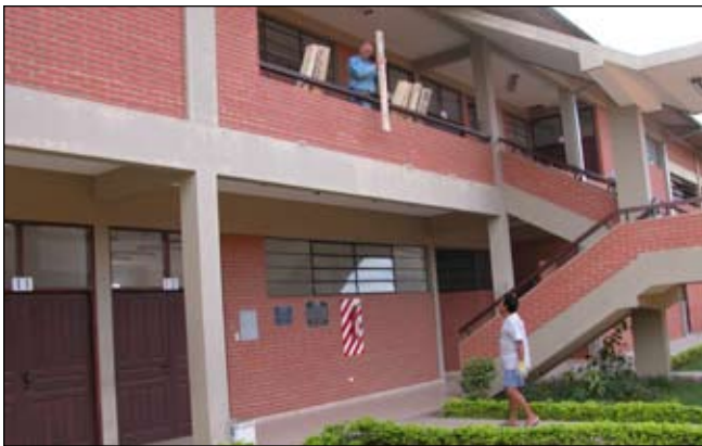
Figure 8—Board being dropped onto concrete walkway as a shock treatment.
