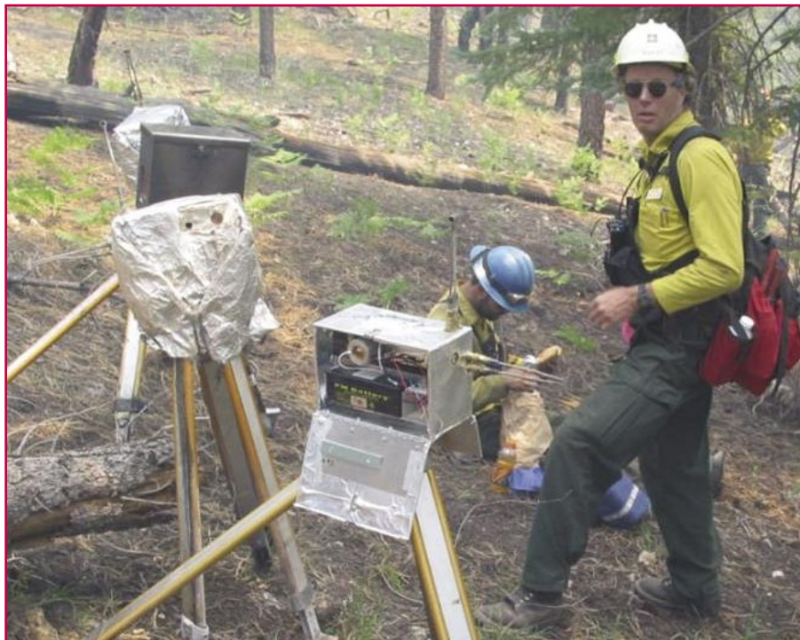
Feel the Heat—Fire-proofed video systems and instrumentation for measuring heat flux, fire behavior, and local weather are installed on the Dragon Complex Wildland Fire Use Incident on the North Rim of the Grand Canyon, AZ, by mechanical engineer Jason Forthofer (sitting) and project leader Colin Hardy. Both men are from the Fire Behavior Research Work Unit, Missoula Fire Sciences Laboratory, Missoula, MT. Photo: Dan Jimenez, Forest Service, Rocky Mountain Research Station, 2005.
