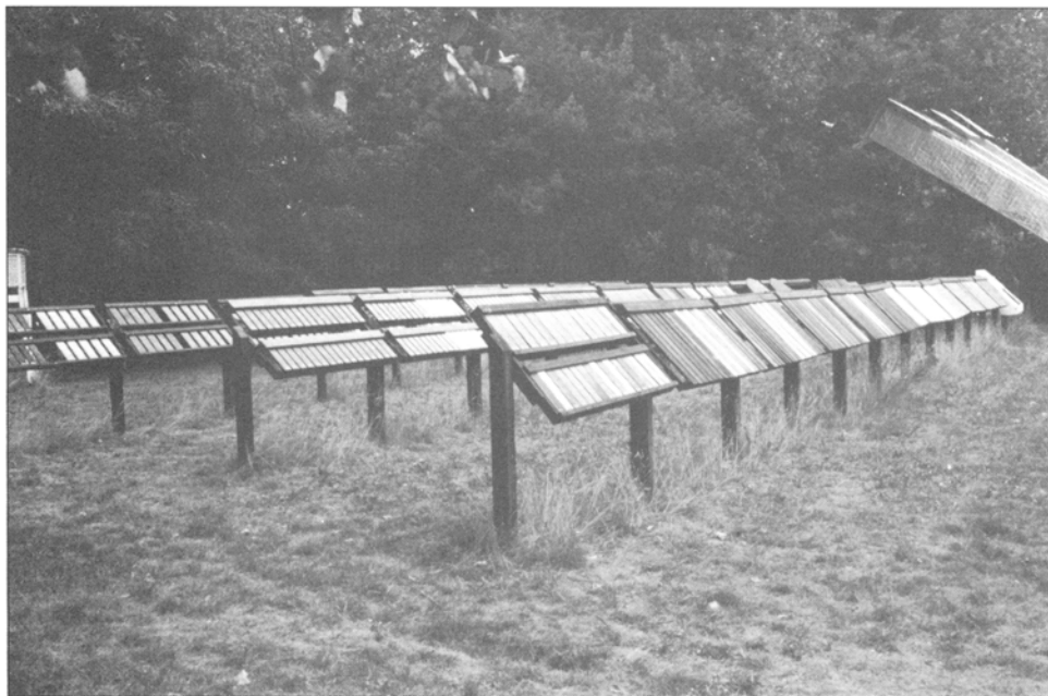
Figure 27 -Durability test of different species at the Wilhelm Klauditz-Institute (Fraunhofer Society) at Braunschweig. (Courtesy of P. Böttcher)
