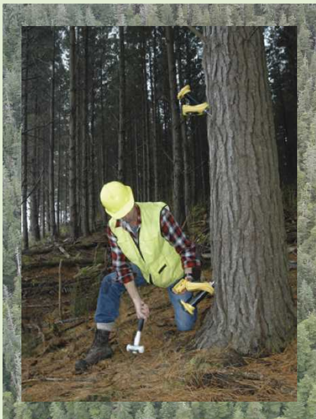
Figure 6. — Assessing wood quality with a portable acoustic tool in forest. (Photo courtesy of Fibre-gen, Inc.)
