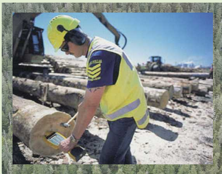
Figure 3. — The use of a hand-held acoustic tool for evaluating logs in a log yard. (Photo courtesy of Fibre-gen, Inc.)
