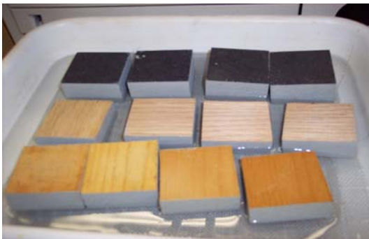
Figure 3. Samples immersed in the water with one side down and sealed sides
