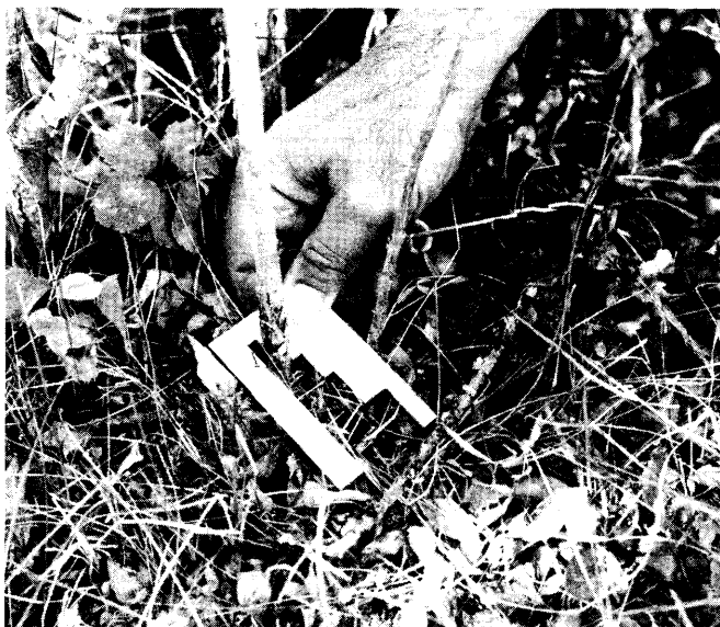
Figure 12.—A go/no-go gage used for tallying the number of shrub stems by basal diameter classes.
