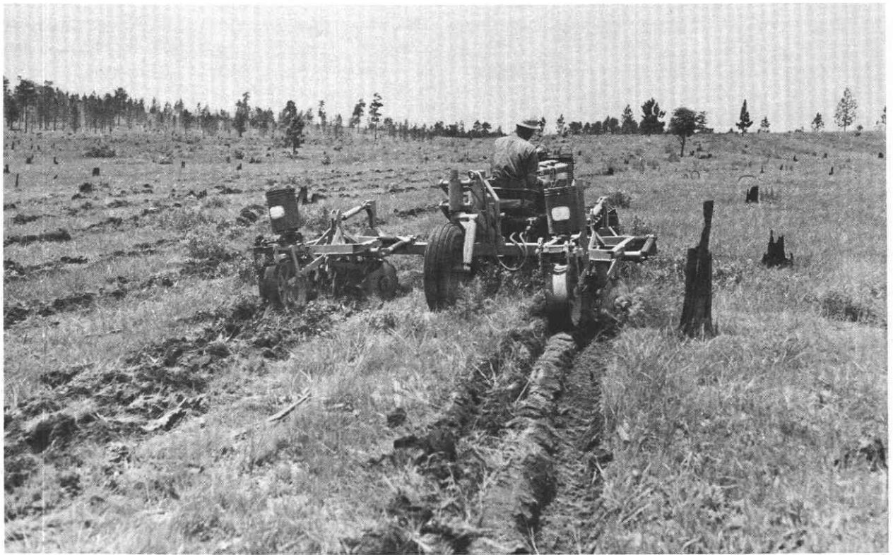
Figure 33.—Disks on this seeder prepare a flat bed.
