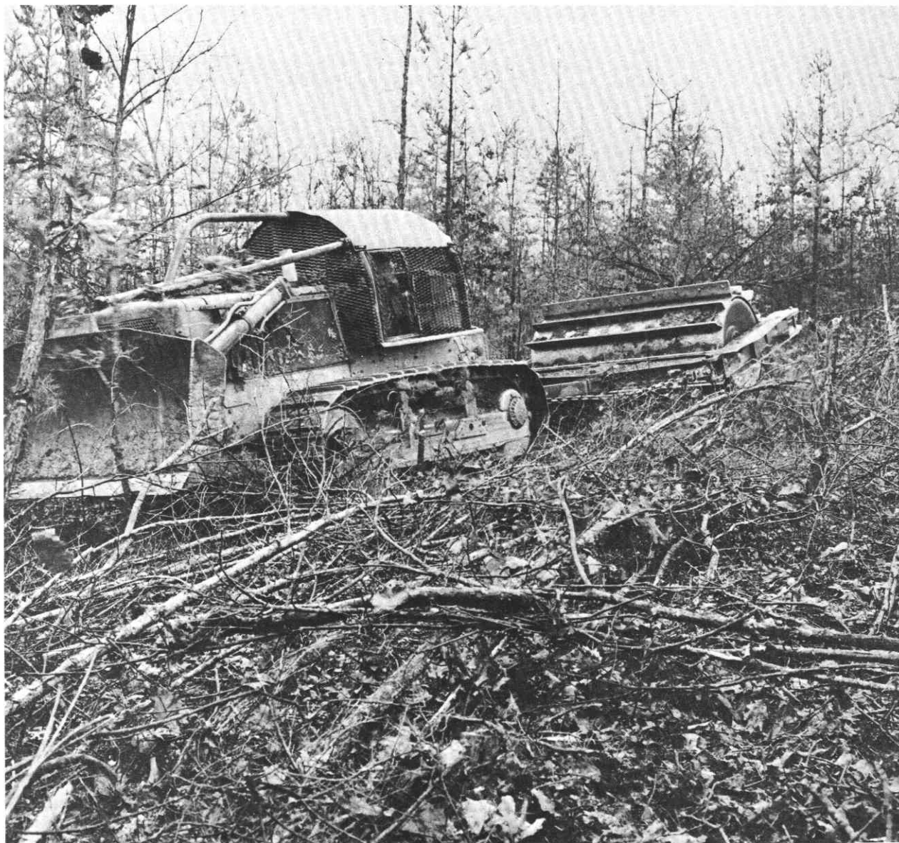
Figure 23.—A heavy drum chopper preparing a site in north Georgia.
