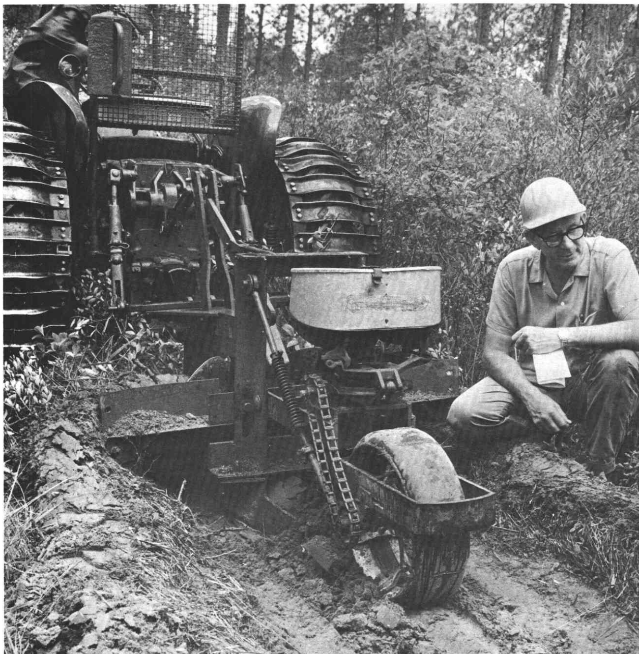
Figure 31.—This row seeder elevates a low ridge in the center of a plowed furrow and drops seed onto it at regular intervals.
