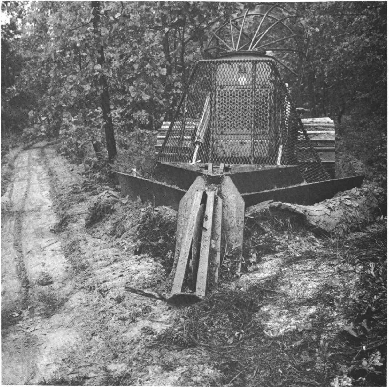
Figure 32.—A front-end row seeder designed for sandy sites and capable of operating in brush.
