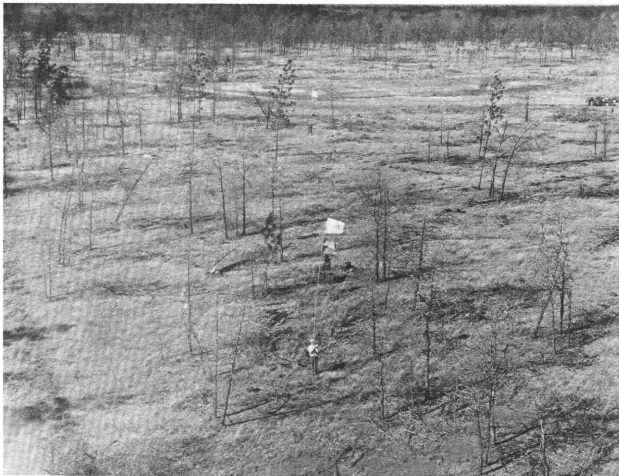
Figure 37.—Flagmen must be placed so that the pilot can align his course on two flags at the start of each flight line.
