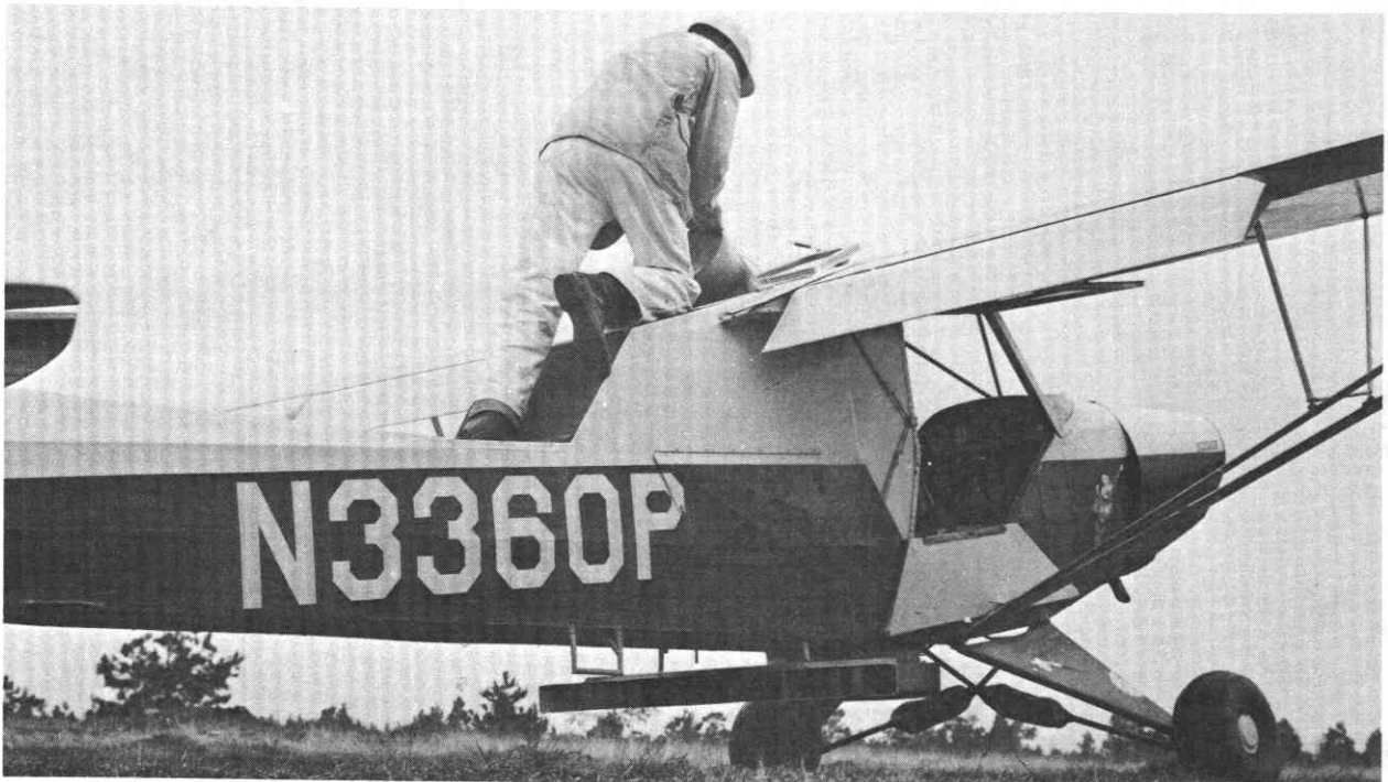
Figure 35.—Up to 1,500 acres per day can be sown from a light airplane. Seed flows by gravity into a distributor that spreads a 66-foot swath.
