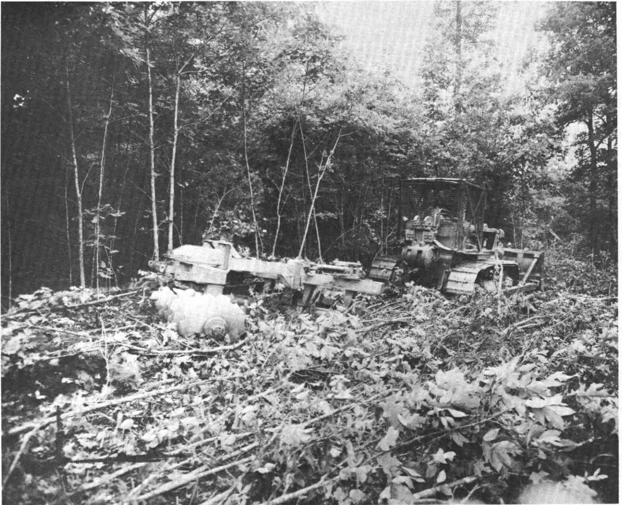
Figure 21.—A 3½-ton disk destroys small, dense hardwood in preparation for direct seeding in Tennessee. (Photo by Tennessee River Pulp and Paper Company.)
