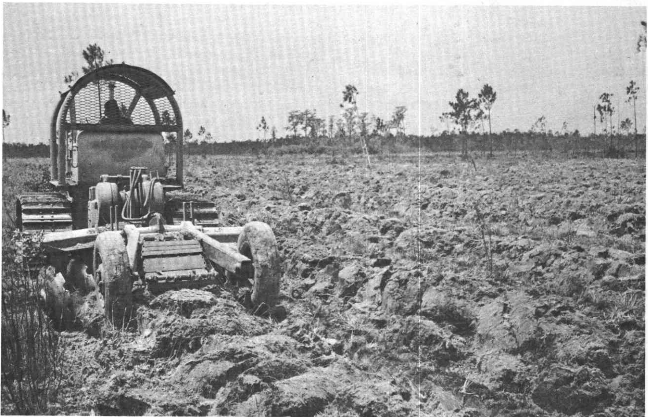
Figure 22.—Disking elevated beds improves tree growth on flatwoods sites with high water tables.
