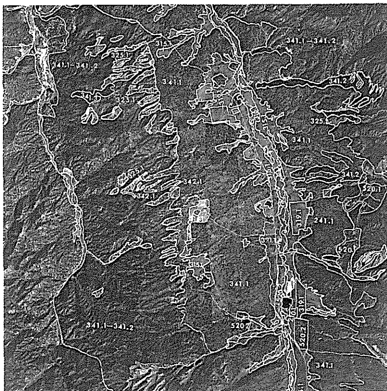
Figure 17—Series classification was attempted in the test of computer-assisted mapping of ERTS scene 1388-17134, August 1973. The ground truth map was made from aerial photography. Some features important to wildland management, the 520 units, are identifiable on the ground truth map but could not be found in the ERTS imagery.
