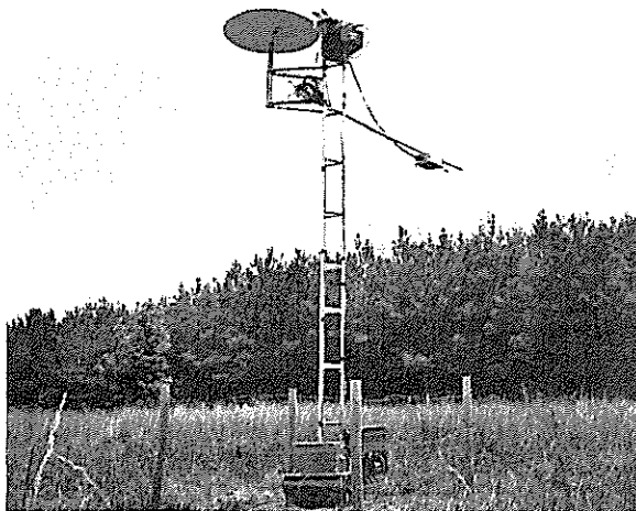
Figure 24—Instruments and equipment for the data collection experiments were set up at four sites within sub-block 2. Shown at the top of the tower ( left ) are the data collection platform (DCP), antenna, incident-energy spectrometer, multiplexer, and light-activated switch. At the end of the 4-m boom arm is the reflected-energy spectrometer. Alkaline battery power packs are at the base of the tower. The interior of a field spectrometer is shown at right .
