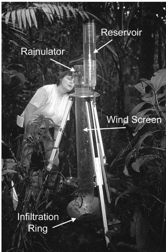
Fig. 4. Photograph of the McQueen rainfall simulator–infiltrometer in the Luquillo Mountains, Puerto Rico.
