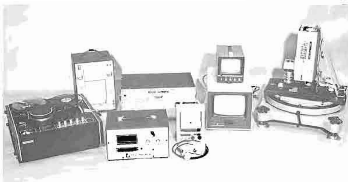
Figure 22—Equipment for aircraft target measurement of terrain reflectance included (left to right) video tape recorder, strip chart recorder, radiometer, static inverter, irradiance meter with input probe and filter chamber, TV monitors, vidicon camera, and radiometer input probe on aerial camera mount.
