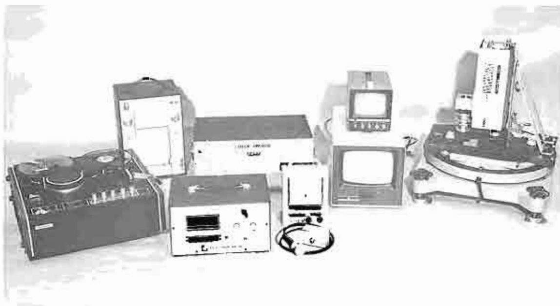
Figure 22—Equipment for aircraft target measurement of terrain reflectance included (left to right) video tape recorder, strip chart recorder, radiometer, static inverter, irradiance meter with input probe and filter chamber, TV monitors, vidicon camera, and radiometer input probe on aerial camera mount.
