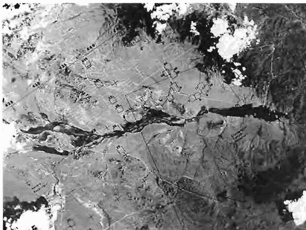
Figure 18—Skylab color photos with sample-square overlays were used for both visual and microdensitometric classification of plant communities at the Region and Series level. In this example (S190B, August, 1:900,000), note the difficulty in discriminating between squares 1 and 2 ( center ). On the ground, square 1 was identified as Shortgrass and square 2 as Mountain Bunchgrass. The overlap between the two squares forms an ecotone between the two classes along a ridge. Square 39 ( lower center ) is a typical Mountain Bunchgrass site at a higher elevation. Two Wet Meadow sites (WM) can be seen left of center. The area imaged is South Park.
