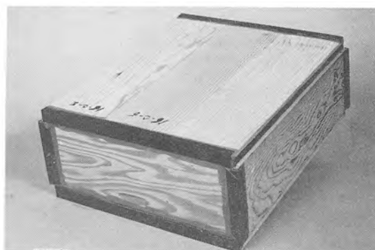
Figure 11.--Box assembled with rubber-base contact adhesive and extruded rubber angles.
