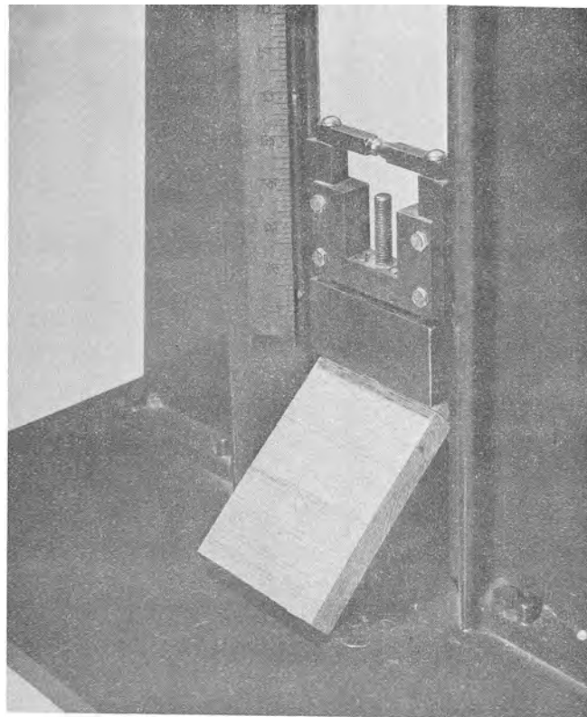
Figure 4.--Impact spread specimen in position shows manner in which impact head strikes apex of specimen.
