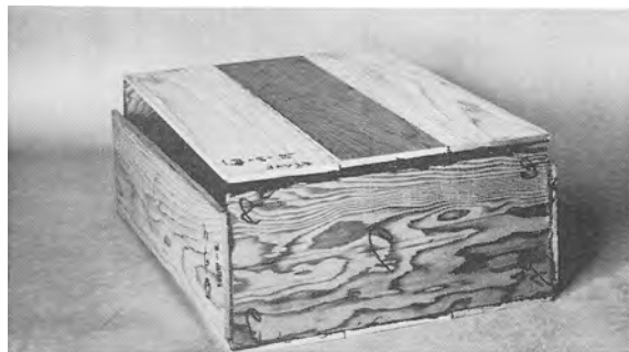
Figure 15.--Example of adhesive-assembled box shows relatively little permanent racking and some joint separation, sustained during diagonal compression test.
