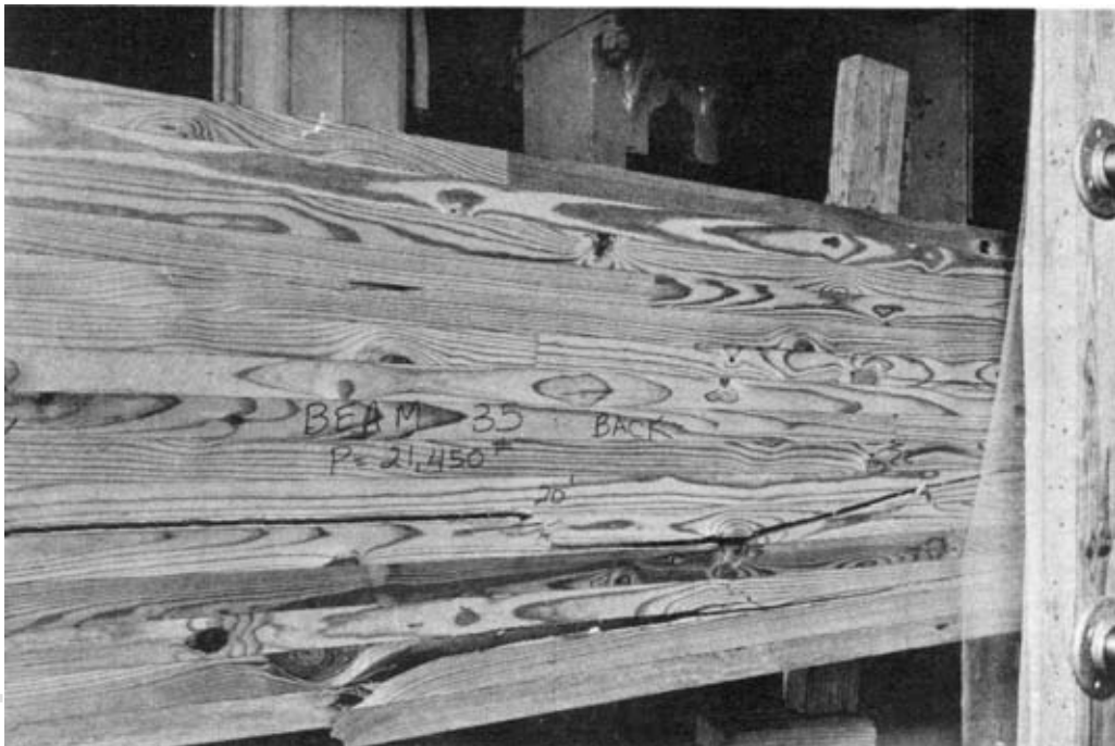
Figure 7.--Failure of beam 35 was attributable to knots rear the edge of the beam in the tension lamination and an edge knot and associated grain deviation in the second lamination. Not shown is a knot in the tension lamination near the opposite edge and about 2 feet to the left of the other knots (see fig. 5). The low modulus of rupture of this beam (3,830 p.s.i.) was attributed to the combined effect of these three edge knots. M 135 719
