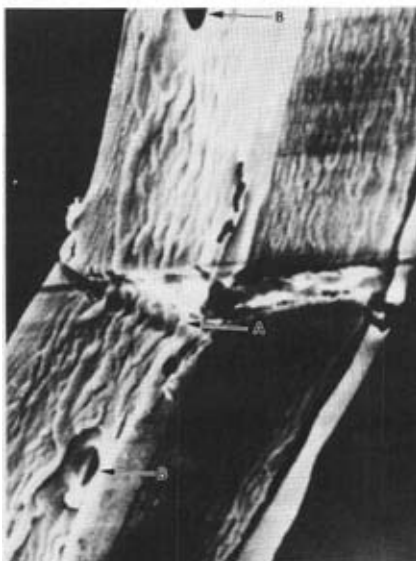
5. Most of the dislocations occurred between bordered pits (Magnification = 2000X). Arrow A shows dislocation situated between the bordered pits indicated by Arrows B.
