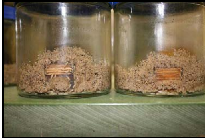
Figure 3. Laboratory termite resistance tests based on AWP A E1-06 standard method (AWPA 2007a)
