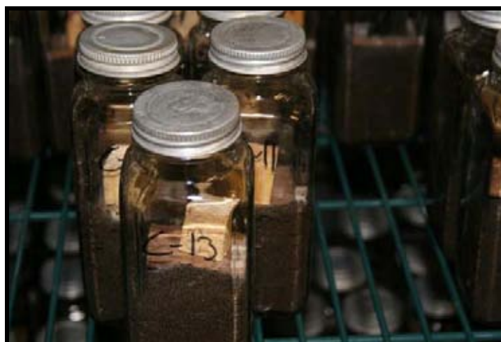
Figure 2. Laboratory decay resistance tests based on AWP A E10-06 standard method (AWPA 2007b)
