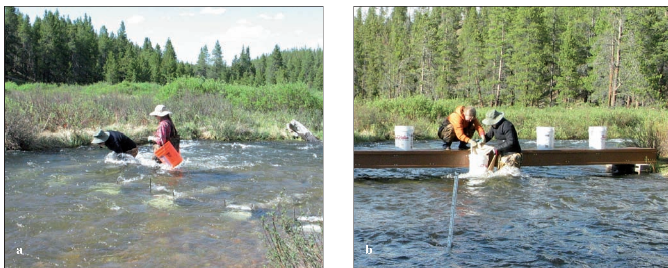
Fig. 2 a and b: Six bedload traps installed in the stream are emptied at 80% of bankfull flow (a). Emptying of bedload trap from a foot bridge (b).
