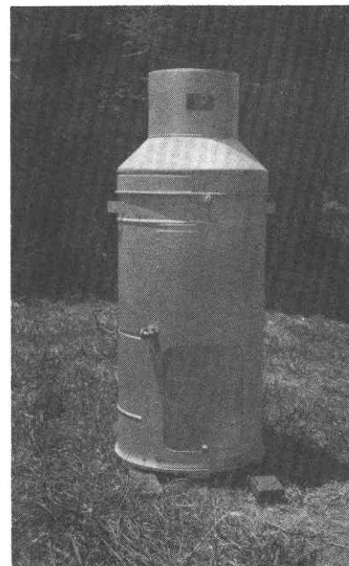
Figure 2—Instrument shelters and a rain gauge were set up on the Redwood Experimental Forest, Del Norte County, California to record temperature, relative humidity, and precipitation.
