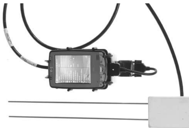
Figure 3 —Components of the TDR nursery soil moisture meter.
