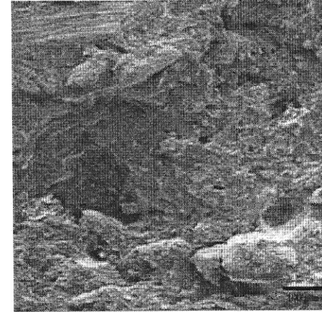
Figure 4. ~ SEM images of PLA-40% PWF: 100 \mu\text{m} (left, 0% silane) and 100 \mu\text{m} (right, 0.5% silane).
