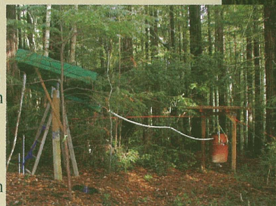
Interception is measured by collecting precipitation inside and outside the forest canopy
