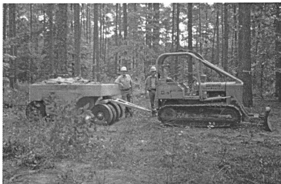
Figure 3. Wobble-wheel road compactor and dozer used to compact soils in the western Gulf Coastal Plain Long-Term Soil Productivity sites. Photo by Allan Tiarks.
