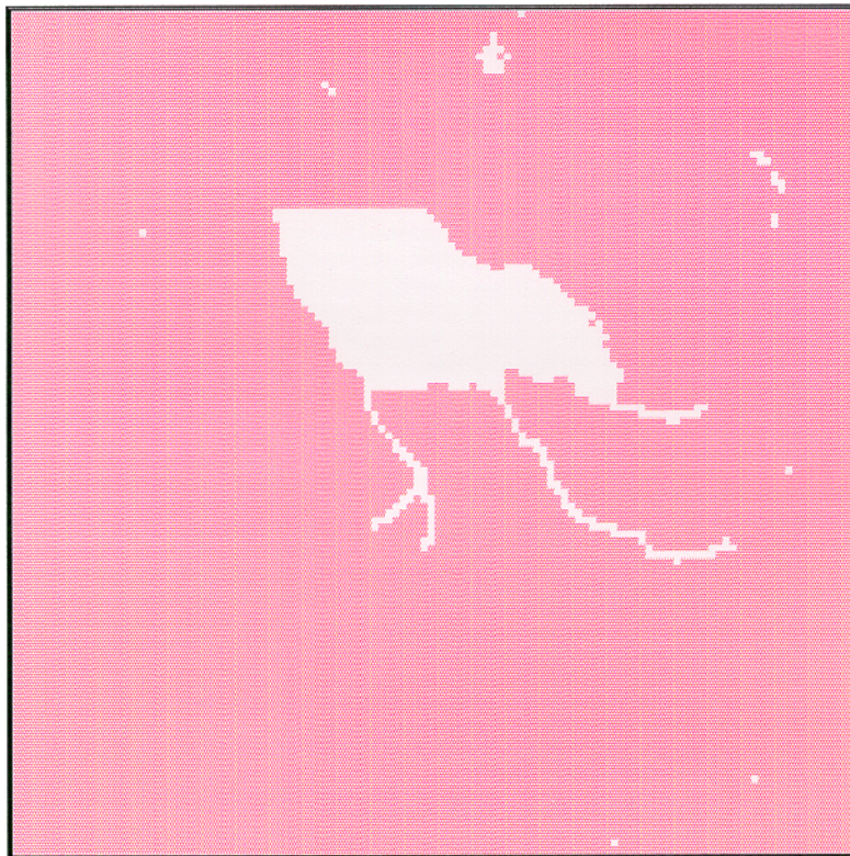
Figure 3-28.—Estimated areas of habitat (red) for the mink (SHG 56) on the Massachusetts study area before and after a proposed development. Note total loss of habitat because of the loss of an extensive block of forested wetland habitat. White represents various wetlands.
