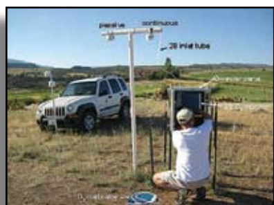
Remote battery powered ozone monitoring station near Silt, Colorado.
