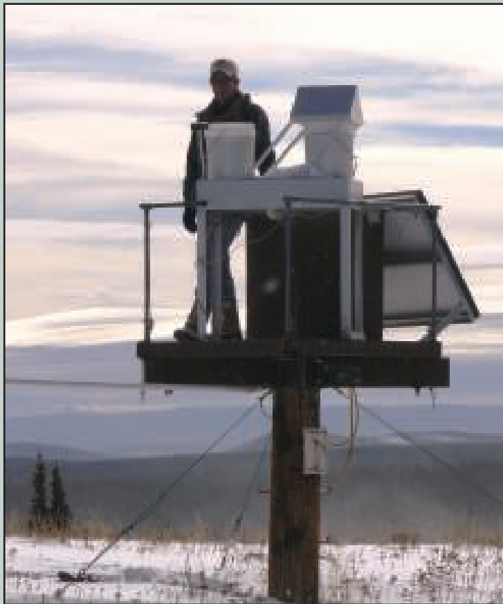
Solar panels power rain and snow collectors at the Glacier Lakes Ecosystem Experiments Site in southern Wyoming. Collected rain and snow samples are later analyzed at a national laboratory for chemical content.
