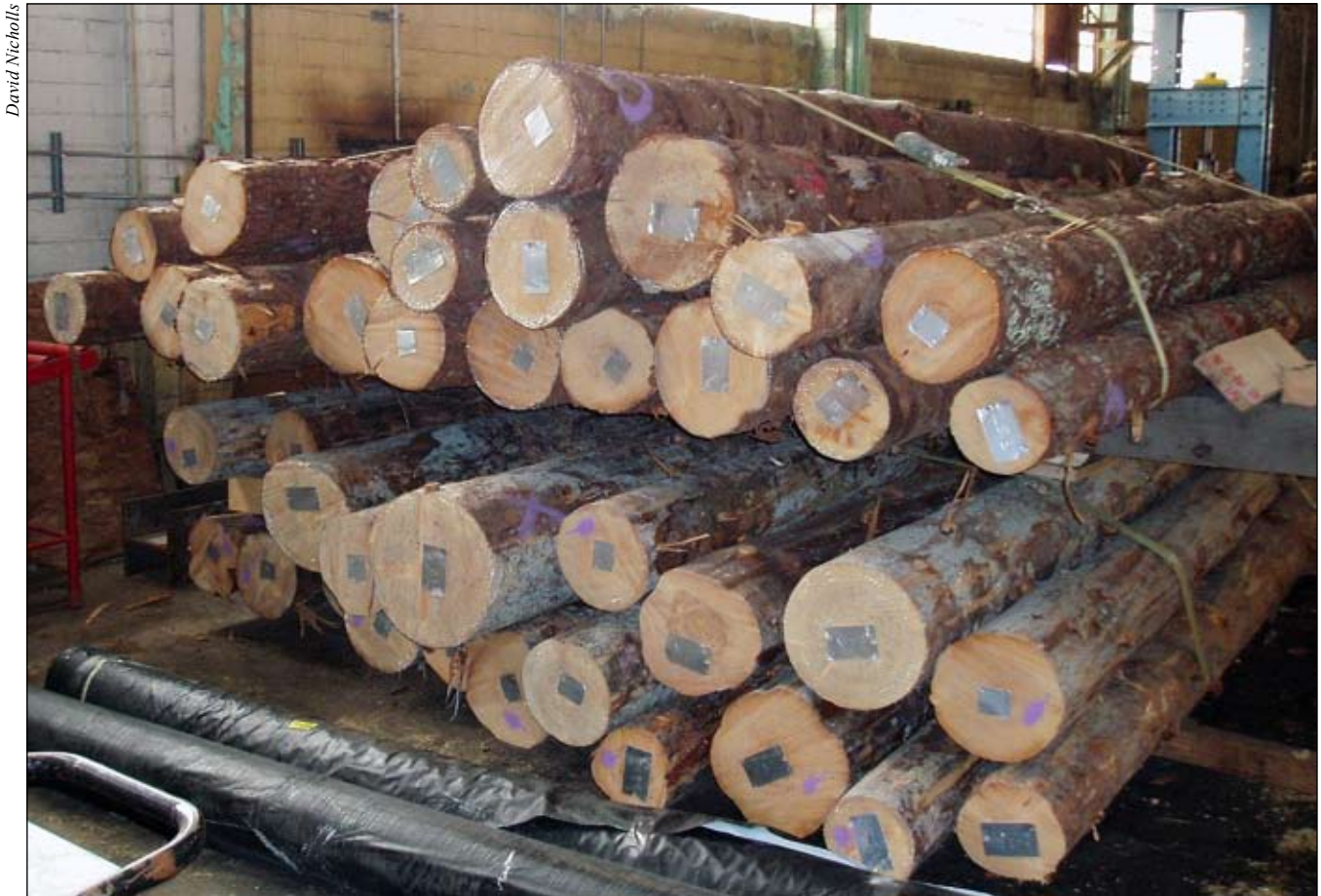
Figure 3—Logs in indoor storage. Identification tags are attached to the log ends.
