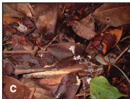
Figure 8. Populus tremuloides (aspen) stakes after about two years of decay outside, at the edge, and at the interior of moist (a–c) and dry (d–f) tropical forest fragments.
