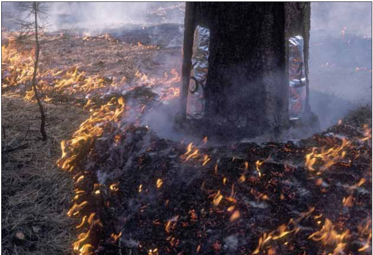
Figure 3. Soil and cambium temperatures being measured during a prescribed fire at Limestone Flats research area where the forest floor material has been removed around the base of the tree.
