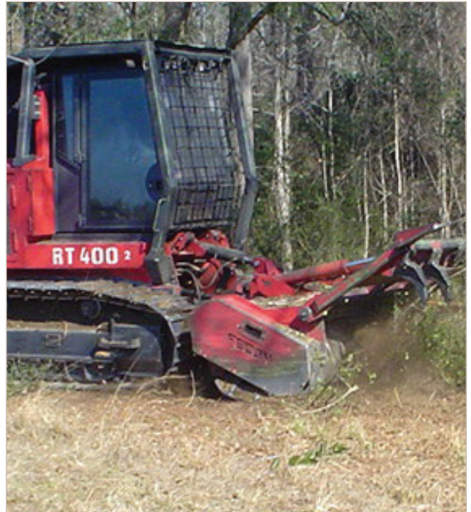
Figure 10—An intense mulching operation at Conecuh National Forest in Alabama with a Fecon RT-400. (U.S. Forest Service photo)
