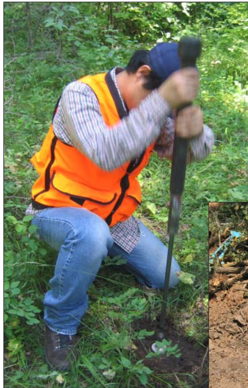
Researcher using an impact hammer core sampler to collect bulk density cores in Northern Idaho. (Photo by Han-Sup Han)
