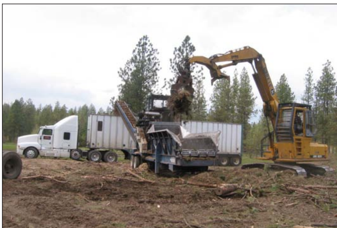
A grinder in northern Idaho reduces biomass to the size needed for use in biomass burners. (Photo by Han-Sup Han)
