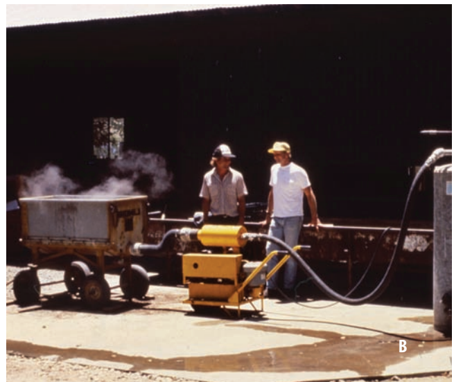
Figure 5.12 —(A) Some commercial growing media have been pasteurized to kill pathogens. (B) For nurseries making their own media, pasteurization with steam or solar heat is simple, effective, and done with portable equipment. Photos by Thomas D. Landis.
