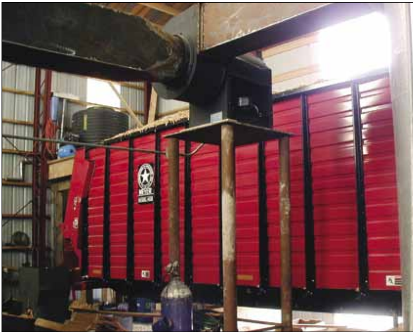
Figure 9—Wood fuel storage bin at Icy Straits Lumber, Hoonah, Alaska.
