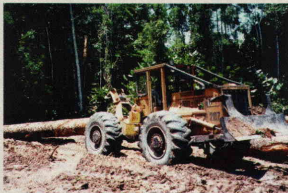
Figure 11 CIB's logging operations all utilize ground skidding equipment such as this rubber-tired skidder, shown here delivering a tropical hardwood log to a roadside landing where it will be loaded onto a logging truck for transport to the company's sawmill.
