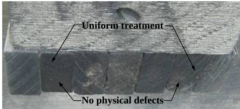
Figure 4-25. Nail laminated deck with individually treated 2x4's on edge showed very good performance and good preservative penetration
