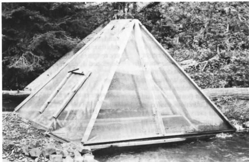
Figure 13.—An adult emergence trap is a modified A-frame anchored to permanently placed wooden beams that parallel the stream.
