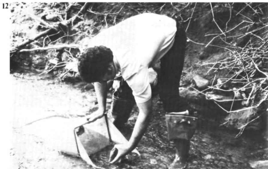
Figure 12.—Surber or modified Surber samplers rely on the current to carry bottom-dwelling insects into a net.
