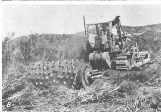
Figure 7.—Preparing brush fuel for prescribed burning: A, Crushing medium brush (mature chamise-chaparral) with the smallest suitable type of bulldozer; B, rolling light brush (chamise-chaparral) to snap as many stems as possible.
