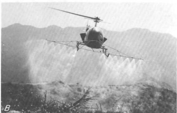
Figure 15.—Two commonly used methods of broadcast spraying to kill brush regrowth: A, Boom mounted on a heavy tractor adapted for spraying in open areas of suitable terrain; B, boom on a helicopter that can be efficiently used on most areas, including rocky or steep slopes, if the areas are of adequate size.
