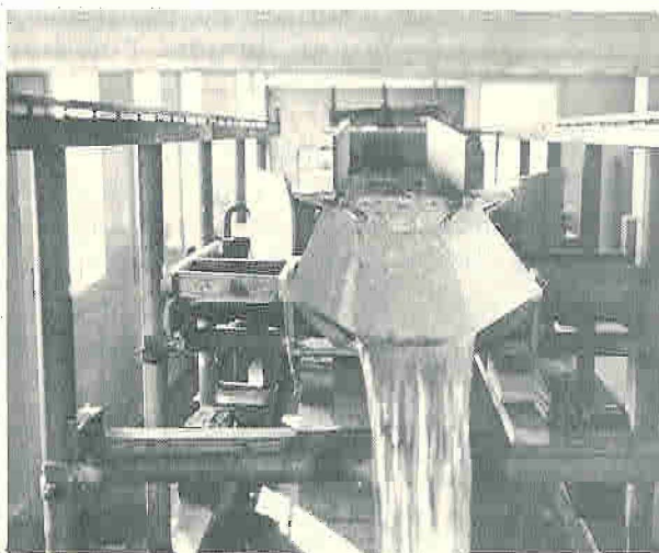
Figure 2.--Typical model flume, with view looking upstream showing model construction and flow conditions in large flume.
