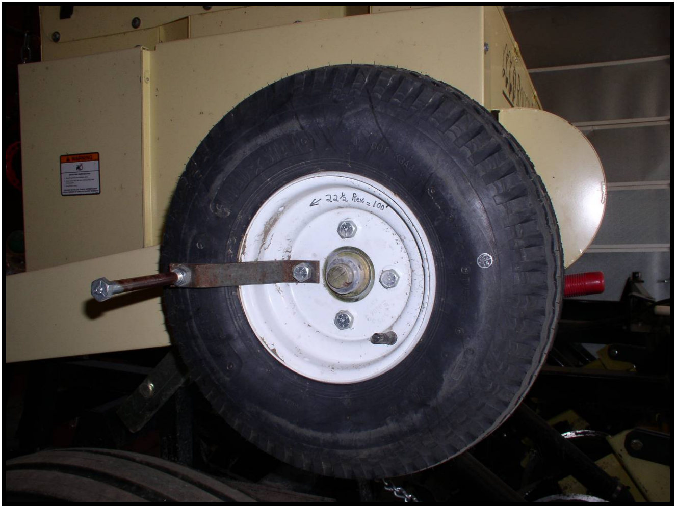
Figure 4. Floating drive wheel with drive handle for calibration, and number of and direction of rotation for drill calibration.
