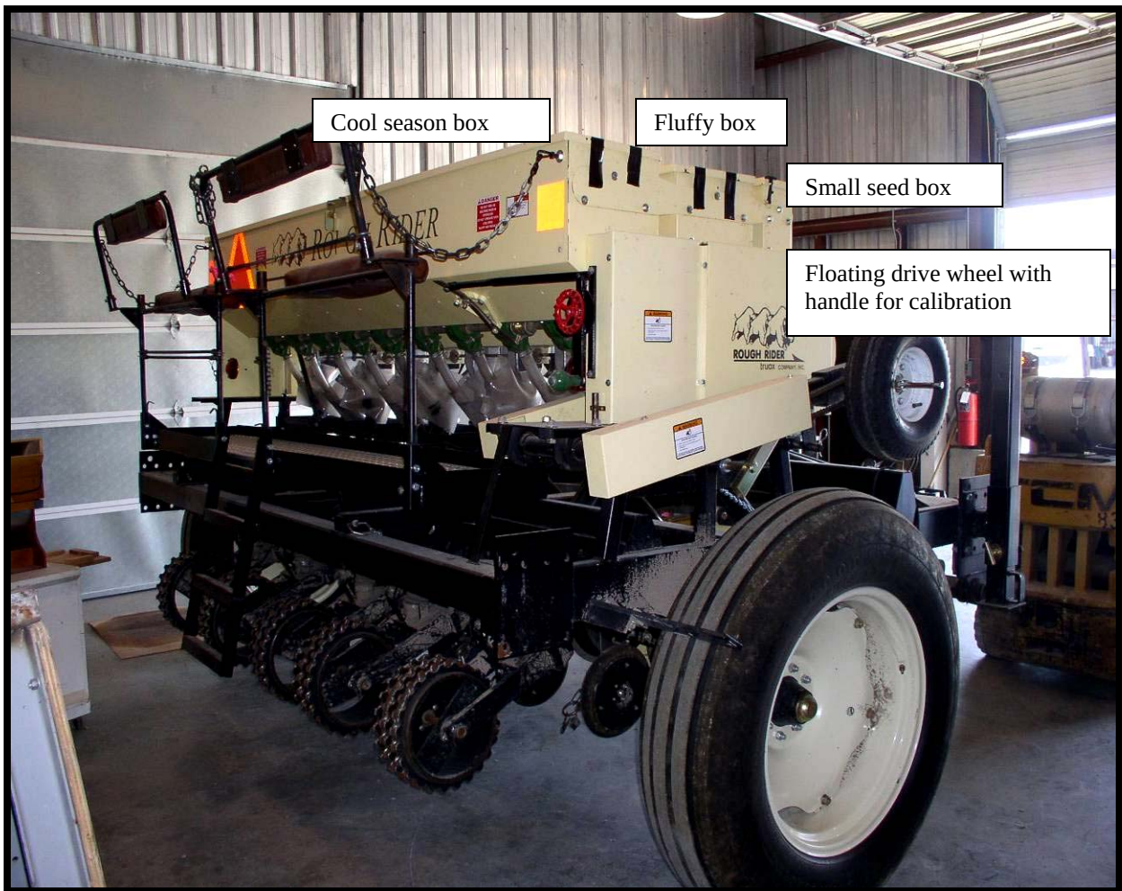
Figure 2. Truax Roughrider seed drill showing location of seed boxes and floating drive wheel with handle for calibration,
