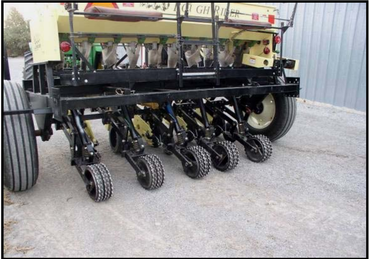
Figure 3. Drill with broadcast planter attachments on alternating rows with drill units.
