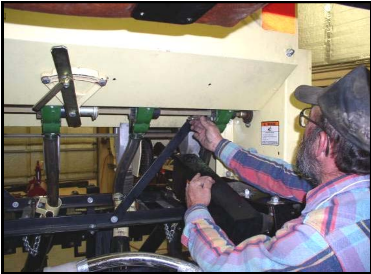
Figure 5. Using a millimeter ruler to adjust openers during drill calibration.
