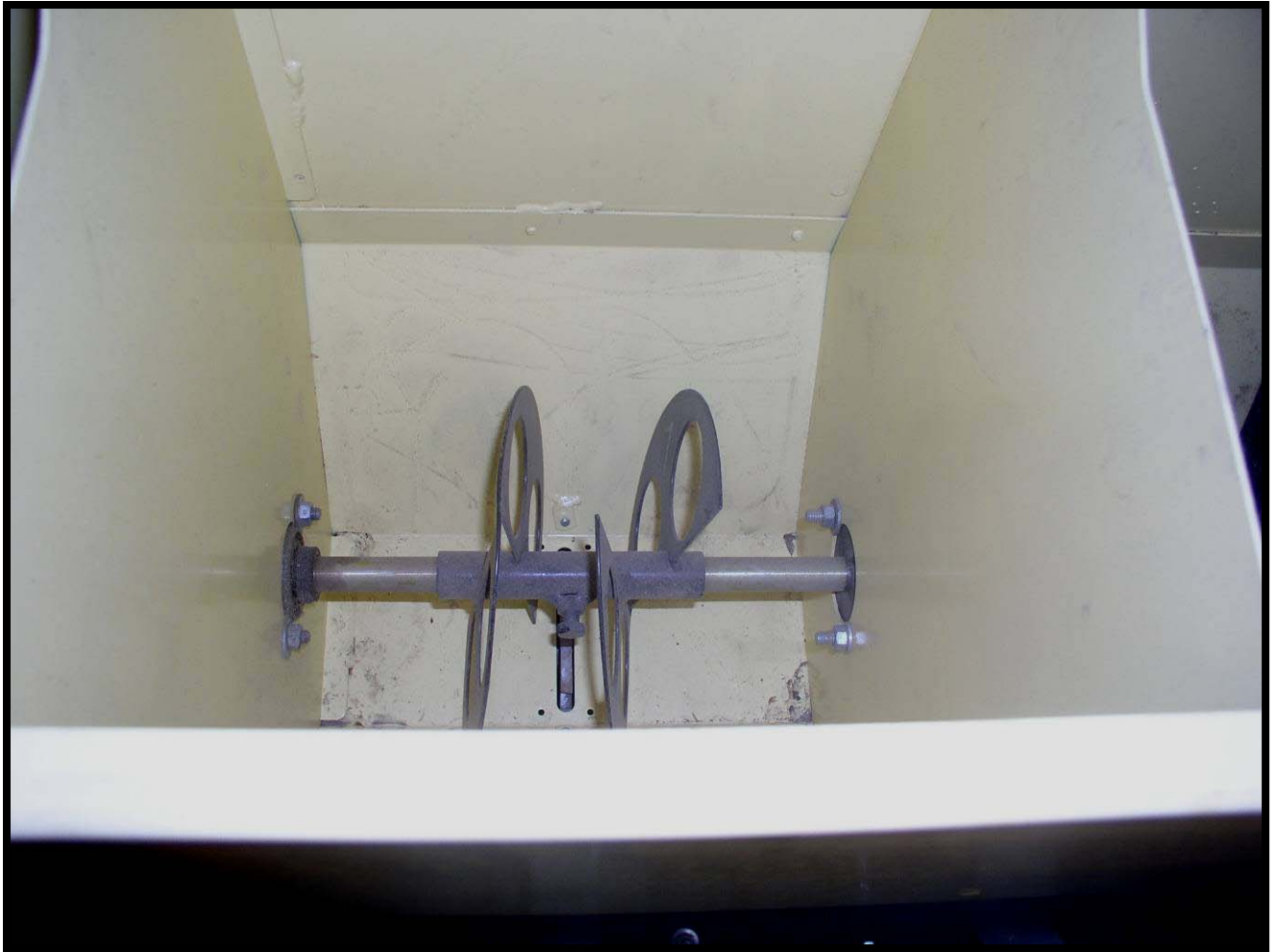
Figure 6. View of inside of fluffy box showing agitator and picker wheel.
