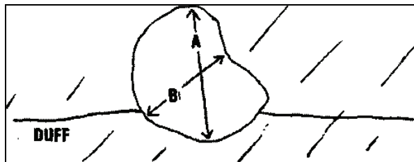
Figure 16.6. This log cross-section illustrates how to measure the diameter of a splintered log. Add diameter A and diameter B and divide by two: (A+B)/2 = average diameter.
