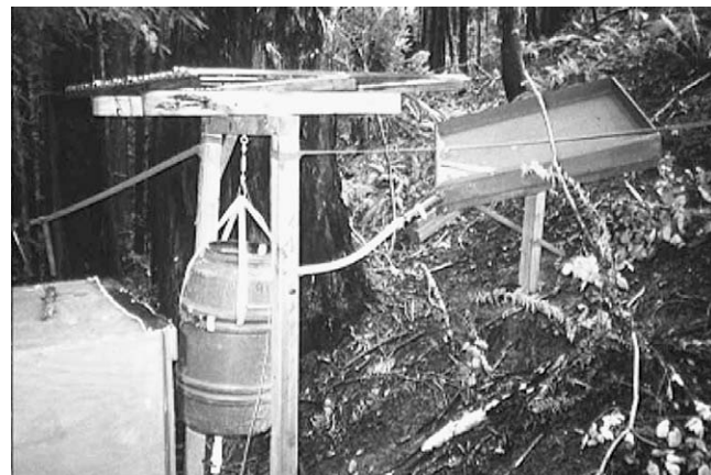
Fig. 1. Throughfall collector (1.2 m × 1.2 m) and plastic storage barrel, which is suspended from a load cell.
