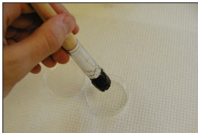
Figure 2—Preparation of “sticky-trap” dust collector.
