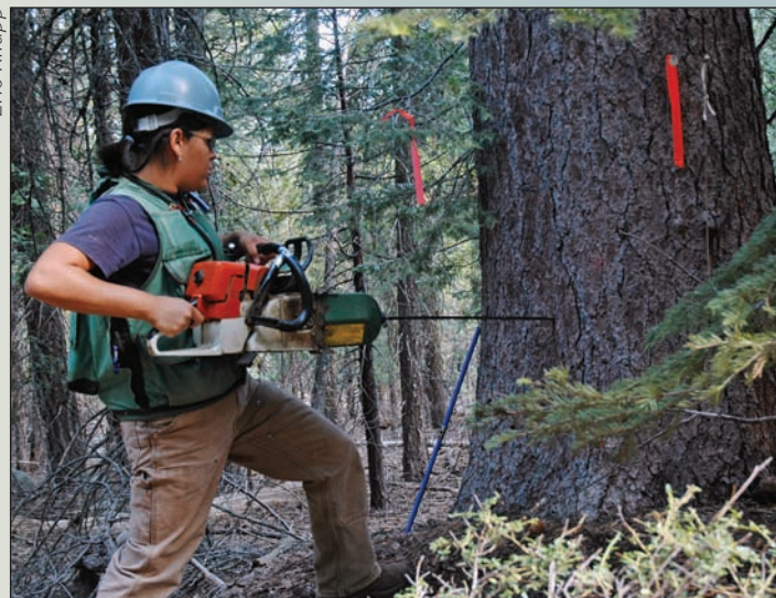
PSW employee Casara Adkins using a chainsaw-mounted increment corer to measure the growth of a sugar pine in response to the 1929 cutting treatment.
