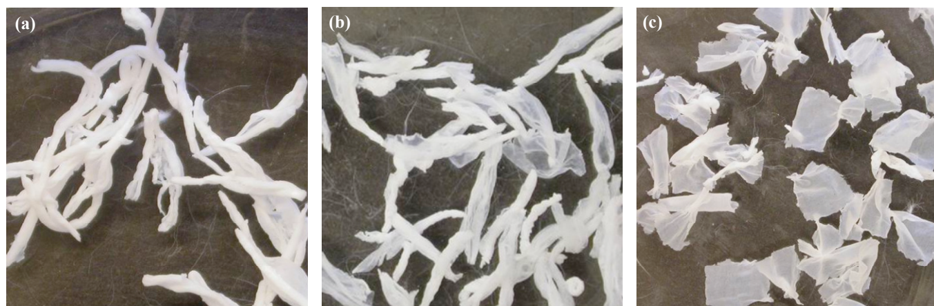
Figure 4. Morphology of adhesive particles after repulping a.) without any additional wetting agent; b.) with 1.75% wetting agent and c.) with 5.25% wetting agent.
