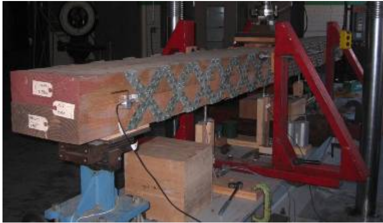
FIGURE 3. TEST SETUP FOR THE LONG (10'-6") 12 INCH WIDE X-BRACED BEAM.
