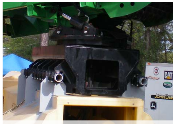
Figure 3. The bundler is fixed to the trailer using two 4" steel tubes.
